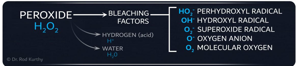
Fig. 8 – As peroxide breaks down/degrades, bleaching factors (most importantly, perhydroxyl radicals) are given off. During this degradation, hydrogen ions (acid) are also given off.
